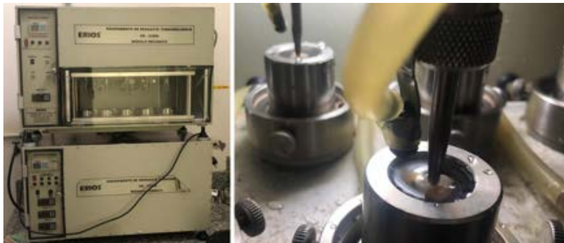
FIGURE 26 A thermomechanical cycling device (ER-37000; ERIOS), in which it is possible to simulate oral masticatory function due to the cyclic load applied to the sample, and also to simulate ageing in the oral cavity with variable temperature promoted by the device
